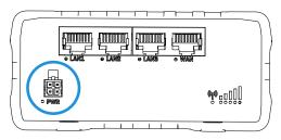
Low-voltage DC power source is used for installations in vehicles, boats and other locations where such a source already exists. This allows you to directly power a device from the vehicle. This is a practical and cost-effective solution that ensures reliability and simplifies the use of power in these locations. You can also power the router by VDC power supply unit (PSU).
